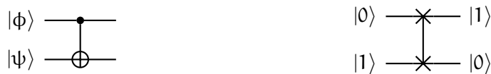
(a) Depiction of a CNOT-gate, corresponding to equation (18) (b) Depiction of a SWAP-gate, corresponding to equation (22)
