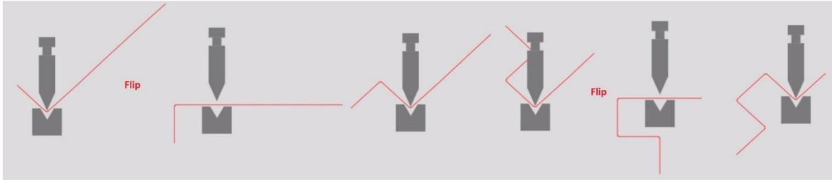
Figure 2.12 Original bending process of an Omega pattern with 2 Flip Operation
