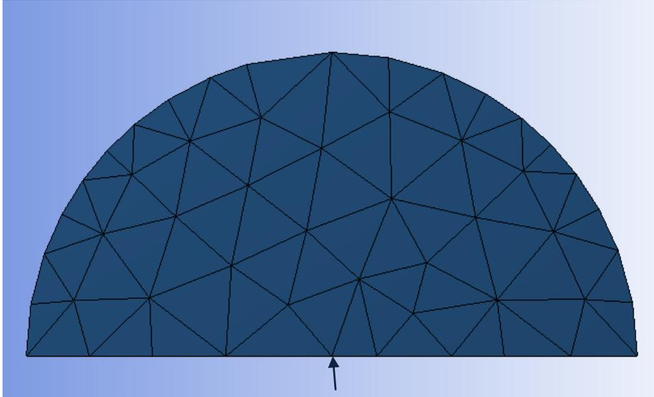
Fig. 3 Semi-circular coarse test mesh
