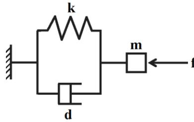
Fig. 1 Scheme of a mass-spring-damper system
