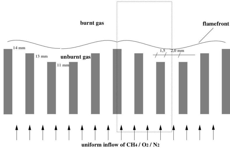
**Figure 3.1:** Geometry of the methane burner; from [Bra98]
