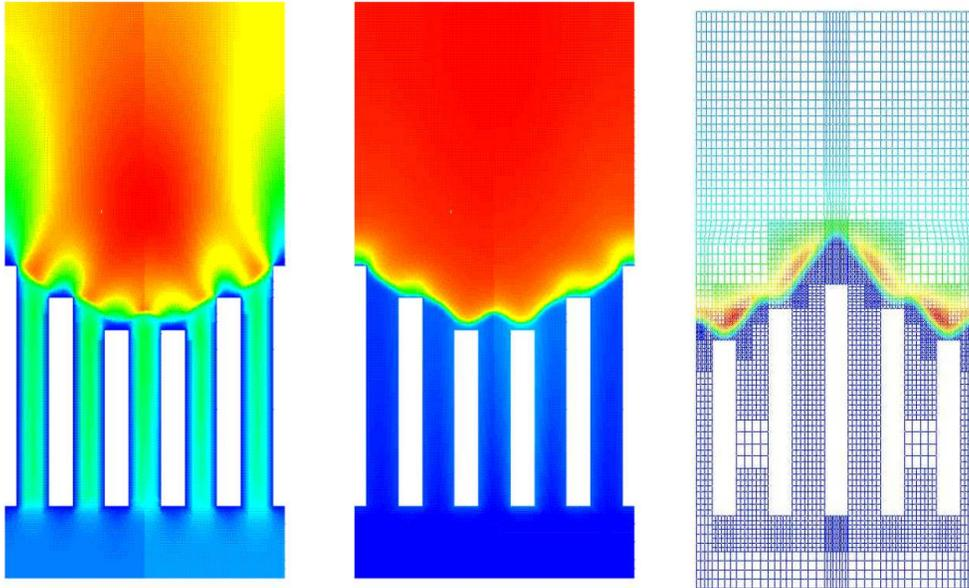
**Figure 3.2:** Simulation results: velocity (left), temperature (middle), mesh with 5000 cells (right); from [Bra98]
